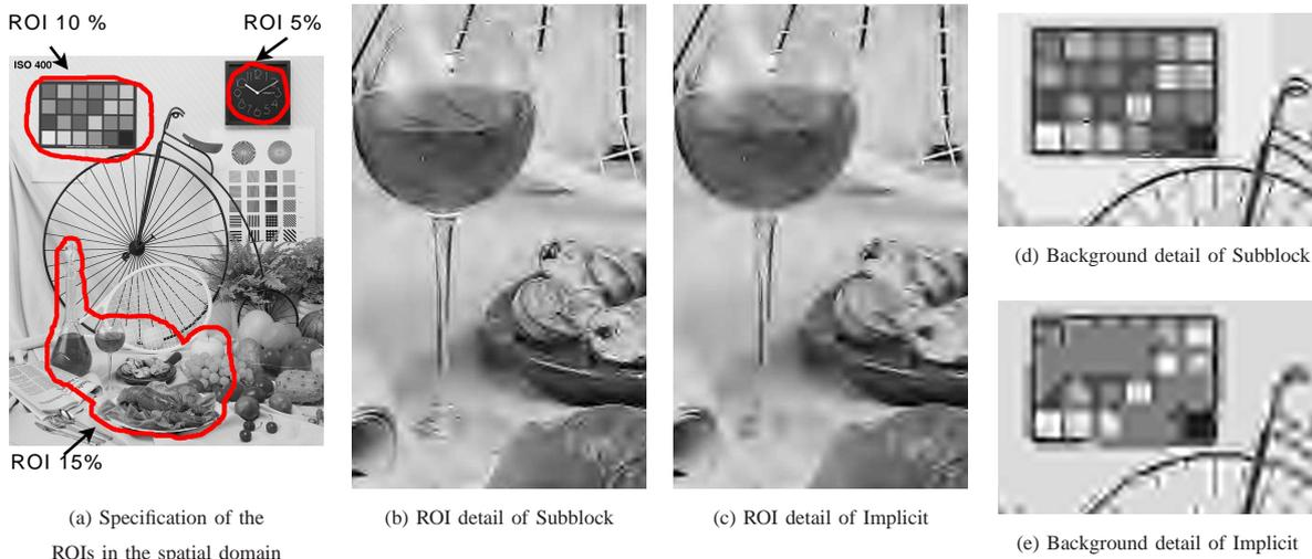
Fig. 3. Visual comparison among the Subblock and the Implicit methods. Bicycle image (size  $2048 \times 2560$ , gray-scaled) with the ROI covering 15% of the image area, encoded at a target bitrate of 0.015 bps. The ROI priority is  $\mathcal{R} = 8$  for all methods.
