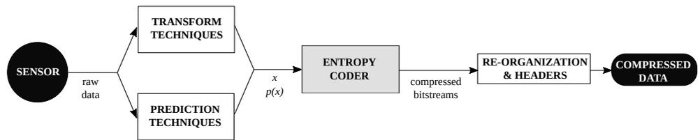
**Figure 1.** Stages of a conventional compression system.
