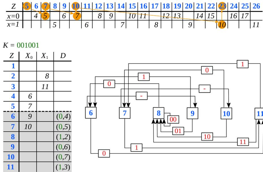
**Figure 4.** Illustration of tANS via asymmetric groups of numbers (top), a tabled automaton (bottom-left) and a state machine (bottom-right).
