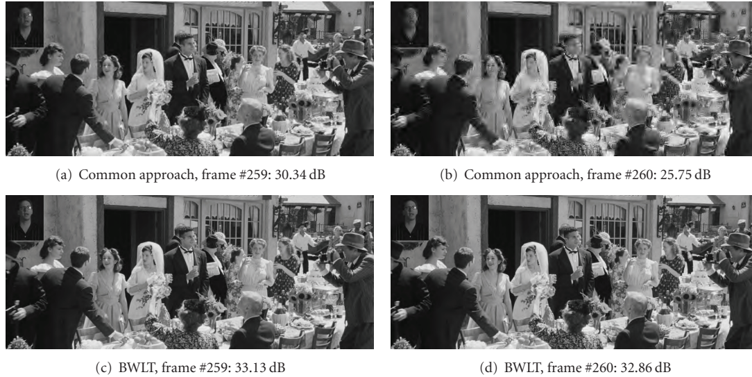
FIGURE 8: Visual comparison between BWLT (c), (d) and the common layer truncation (a), (b) for two frames of the “StEM” sequence. The common truncation produces irregular quality, which leads to flickering.
